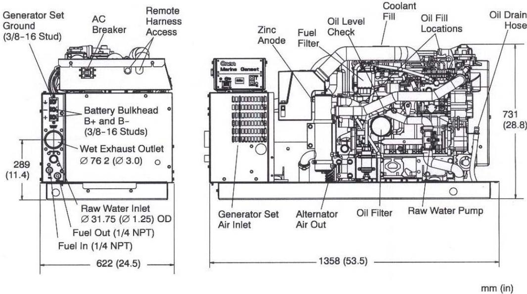
**Note:** This outline drawing is provided for general reference only and is not intended for design or installation. For more information see Operation and Installation manuals or obtain drawing 500-4307 and wiring diagram from your distributor/dealer.
